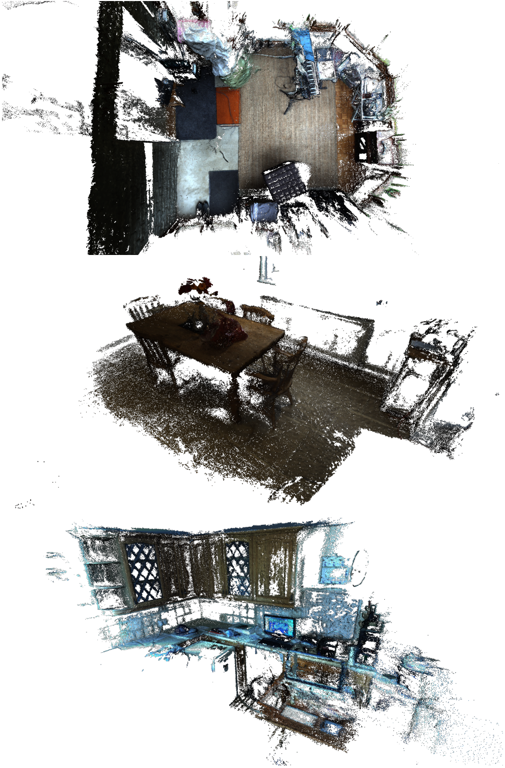
Figure 6.6: Reconstructions made using the reconstruction system outlined in the previous section. We use a coarse-to-fine approach to estimate depth maps and use ORB-SLAM for tracking.
